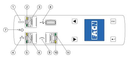
The ePDU front panel includes communication and monitoring ports. LED status indicators, and operation buttons. The ports and the associated LED indicators are described in the following table
